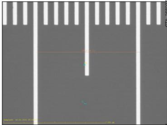
Image of an optical grid with 10 µm bar spacing
