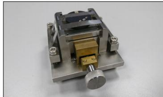
Clamp-type specimen holder
