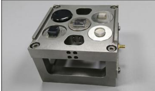
Steel specimen holder for 5 small specimen inserts, Ø 24 mm, insulated upper section
