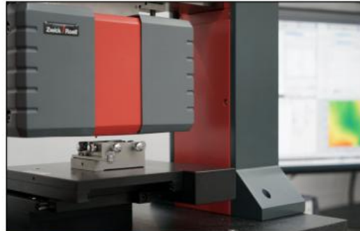
ZHN-S Nanoindenter; detail view
