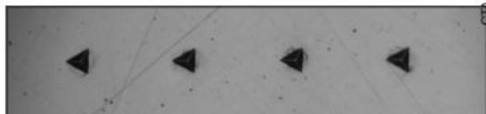
Berkovich indentations with 500 mN in steel and specimen grip position superimposed
